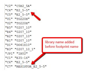
If there is no duplicate footprint warning in the log file, the back annotation process can be skipped. In that case, move ahead to **"Synchronizing OrCAD X Capture and PCB Editor Design"**.
